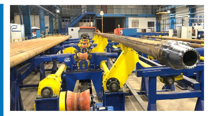
Steady rest loading lines is designed for the piece-by-piece supply of pipes from the pipe rack to the processing position on the lathe, holding the pipe in the steady rest of the line when processing it in the machine, and transferring the pipes to the next pipe rack after the end of turning.
