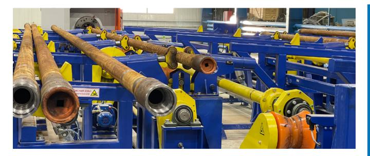
The presence of a pipe in the line is controlled by an optical sensor installed on the steady rest closest to the machine. The lifting / lowering of the roller supports is controlled by sensors that control the end positions of the pneumatic cylinder.
